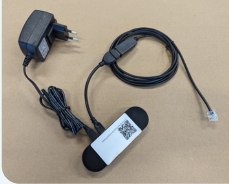
P1 port reading smart meter
