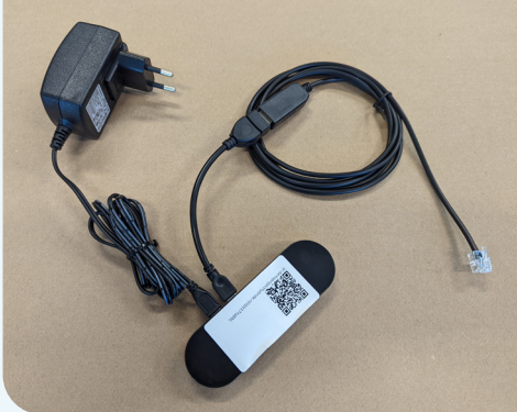
P1 port reading smart meter
