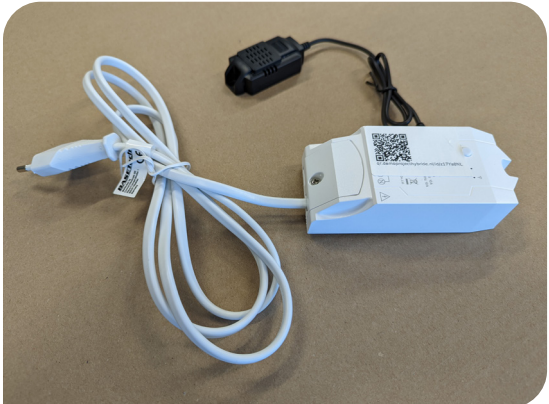
Measuring unit for temperature and humidity in living room
